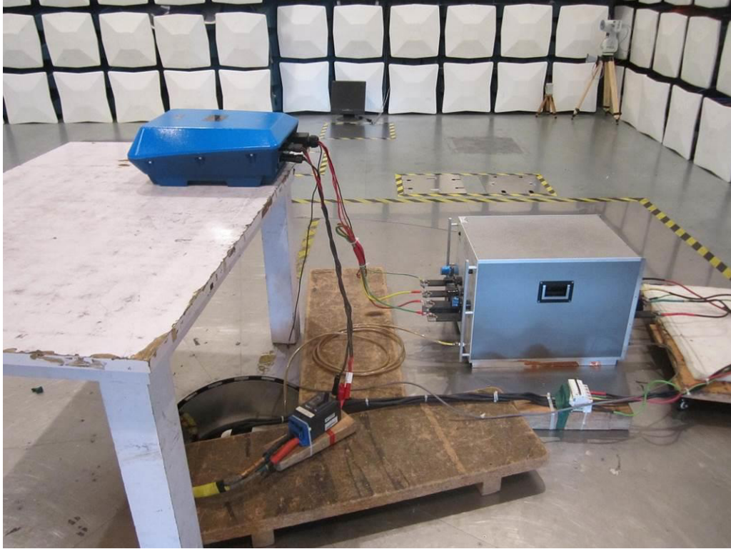
Photograph 1: Set-up for Conducted Emission
