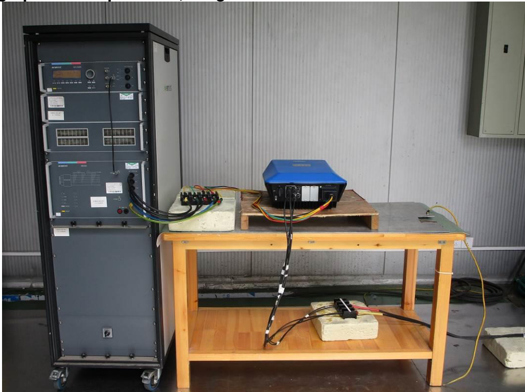
Photograph 6: Set-up for EFT, Surge
