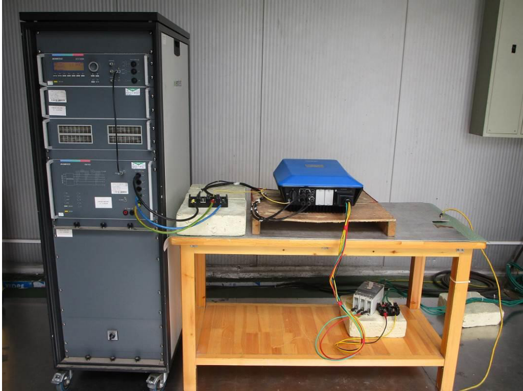
Photograph 7: Set-up for Electrostatic Discharges (ESD)
