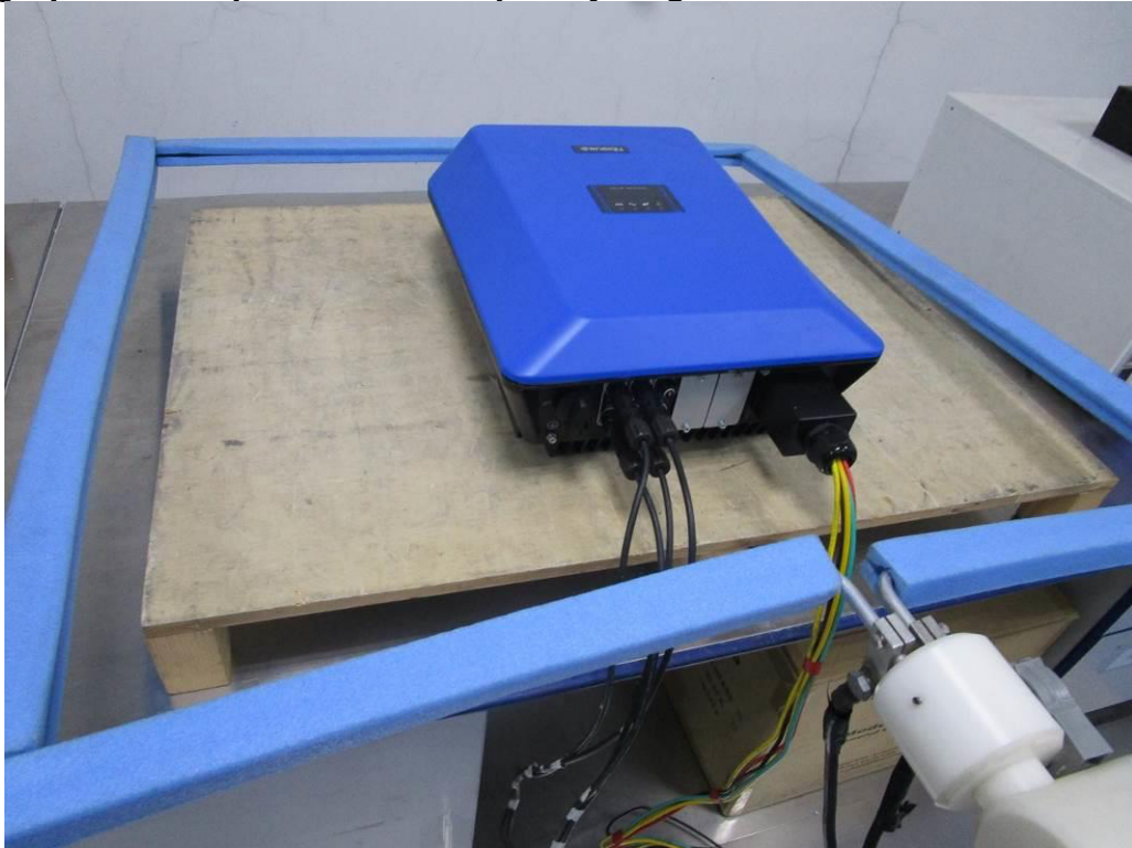
Photograph 6: Set-up for EFT, Surge
