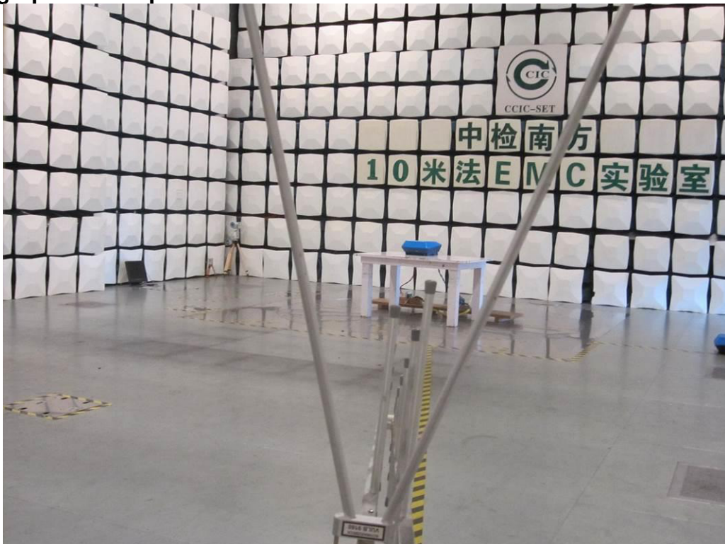
Photograph 2: Set-up for Radiated Emission
