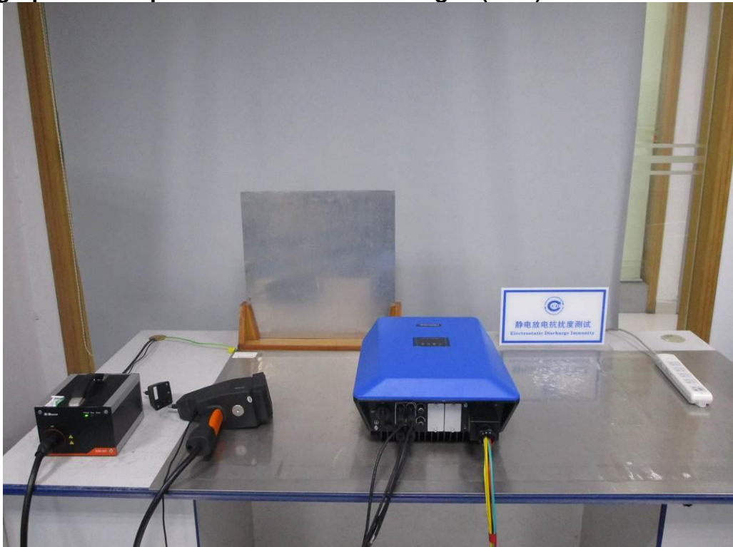
Photograph 7: Set-up for Electrostatic Discharges (ESD)
